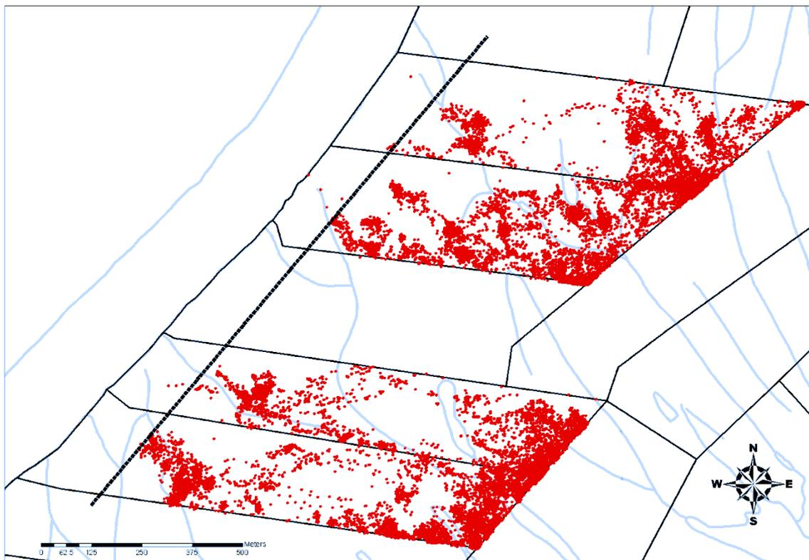
*Fig. 1. Distribution of animals before (top) and after (bottom) the automated animal control devices were activated. The thick line represents the location of the virtual fence line and removes the animal's access to the riparian area.*
