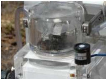
*Fig. 1 Cuvette measuring chamber for CO<sub>2</sub> exchange of cyanobacterial crusts that remains open 90% of the time exposing the crust to natural environmental conditions.*
